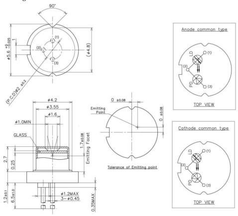
All dimensions in millimeters Unless otherwise specified, Tolerance  $\pm 0.3$ mm
